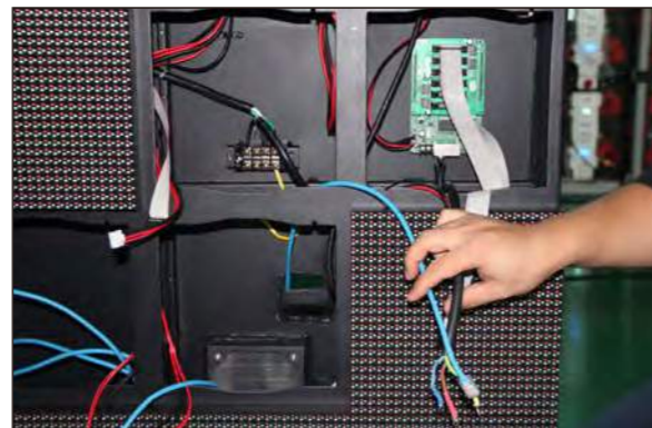
Step 6: Open the module and find the net and power cable
